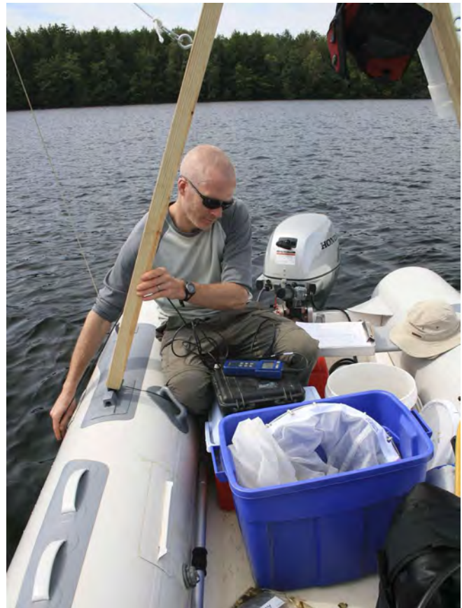
Top: Motorboat used during the study. Bottom: Ethan taking a vertical temperature and dissolved oxygen profile using the YSI.
